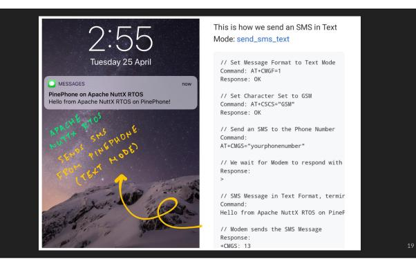
And here are the AT Commands For sending an SMS Text Message
