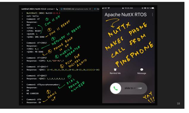
Here we see the AT Commands Sent by NuttX to the LTE Modem For making a Phone Call
